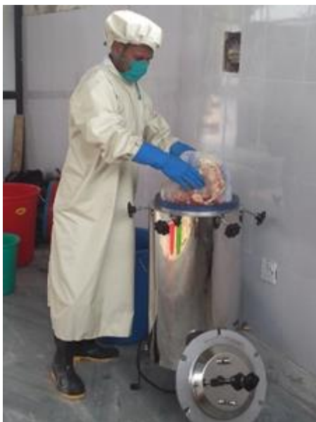
Picture 10: Treatment of infectious waste in an autoclave
