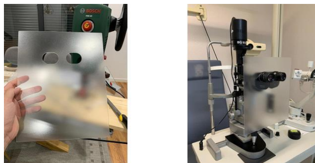
Figure 2: Creating a Slit Lamp Barrier
